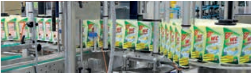
One of the four new high speed filling lines installed in Strzelce, filling acid based toilet cleaners.
